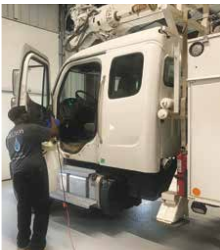
ON THE JOB: Mike Hardy, Bailey’s Zero Hazard, treats the interior of a bucket truck at the Shippensburg District truck garage with hypochlorous acid, a non-toxic chemical disinfectant.
